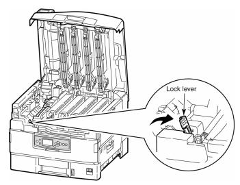
4. Grasp the fuser handle and lift the fuser out of the printer. Dispose of it in accordance with local regulations.
